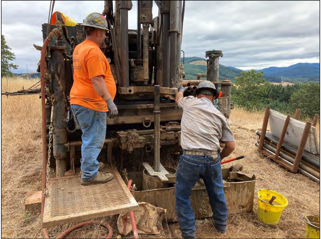
Drilling was performed using hollow-stem auger, mud-rotary, and HQ wireline coring techniques.
