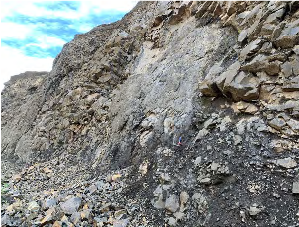
Photograph 2. Steeply dipping joint trending subparallel to an existing cut face.
