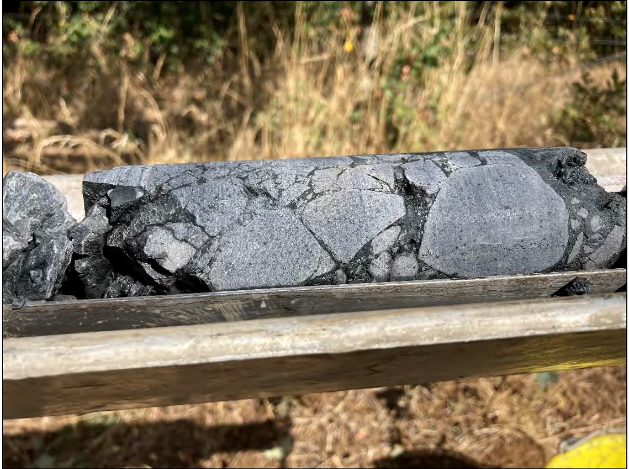
Typical rock core, consisting of brecciated and altered basaltic rocks of the Siletz River Volcanics.
