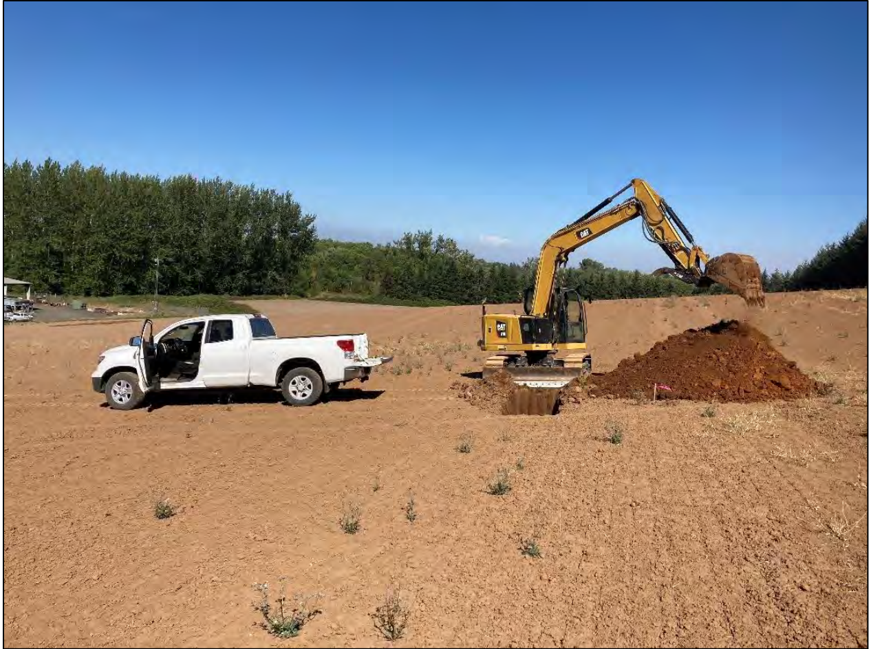
Test pits were advanced to the limit of the machine's reach, or excavator refusal on competent bedrock.
