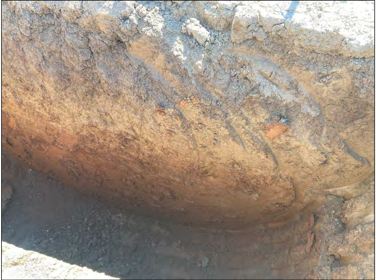
Typical test pit profile, consisting of weathered in-place volcanic soils transitioning into bedrock.
