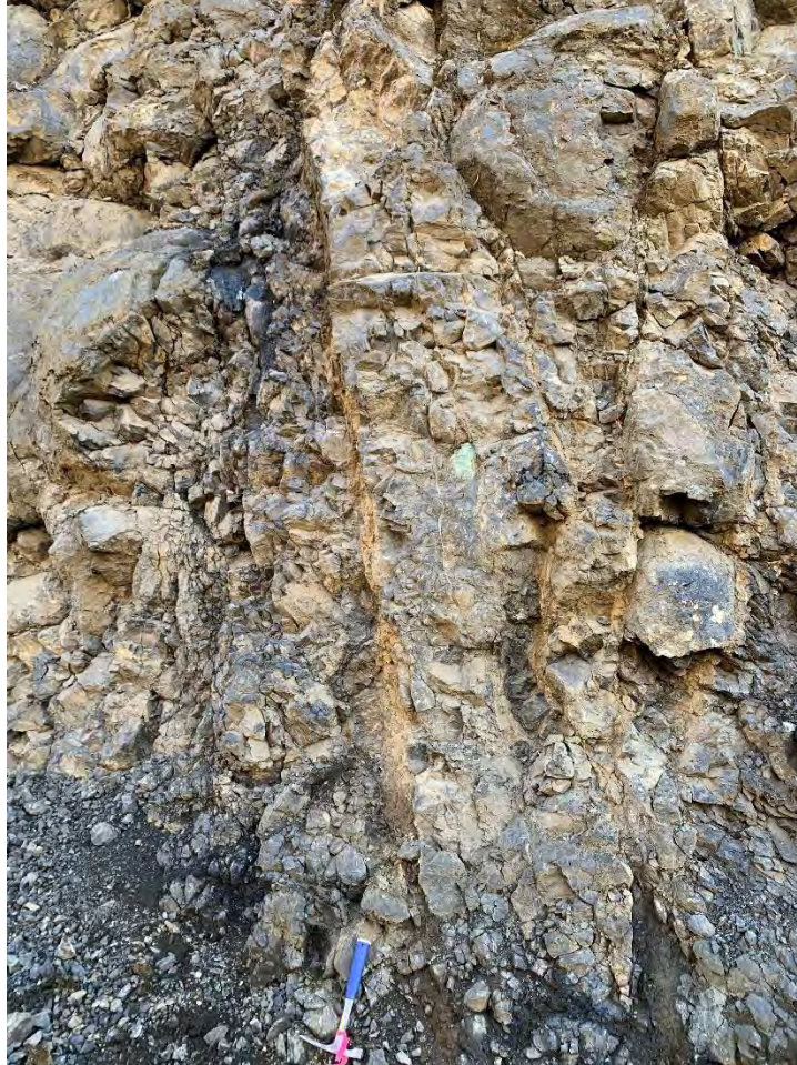
Photograph 1. Typical steeply dipping joints in the existing Coffin Butte quarry.
